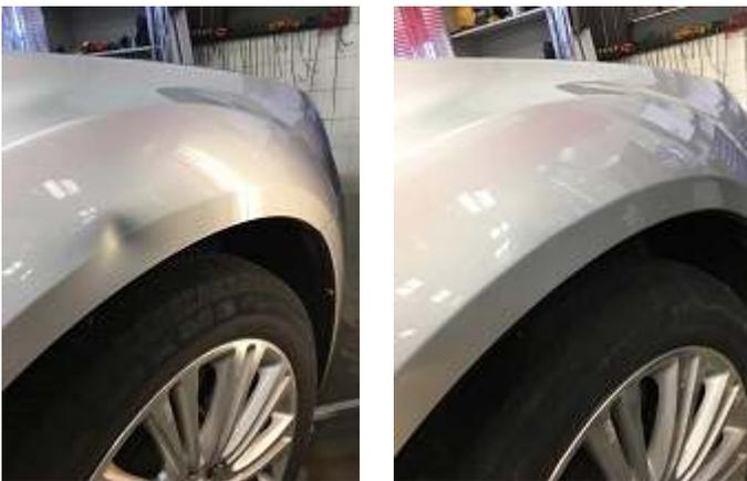
*Paintless dent repair shows dent in left photo; right photo shows the results of the repair.*
